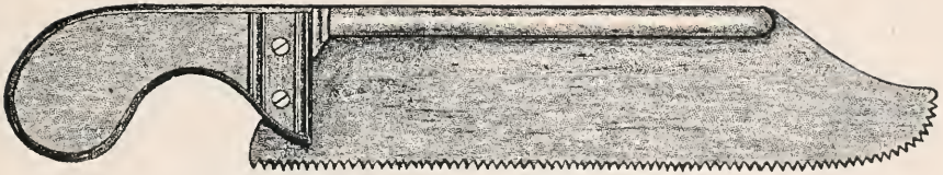
FIG. 22.—A very desirable saw for post-mortem work; it is solidly constructed, and the teeth on the curved end are useful for sawing out the angles in the removal of the skullcap by the angular method. (Slightly less than one-half natural size.)
